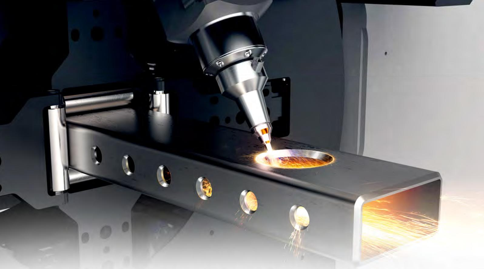
**NEUER ROHRLASER MIT BIS ZU 220 Ø**
